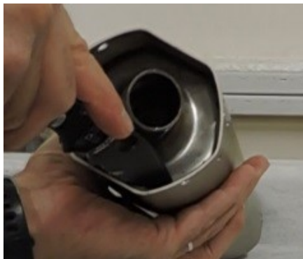
Figure 1- Scoring sealant around Packing Stop Plate.
