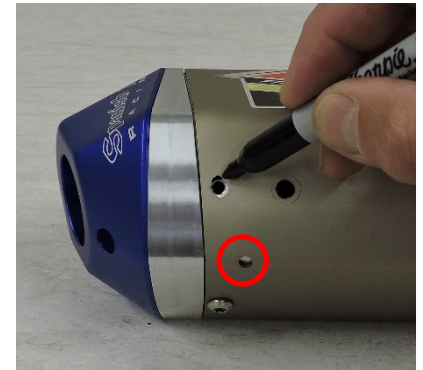
Figure 3- Marking location where Cab hole needs to be enlarged.
