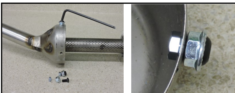
Figure 2- Installation of press in nuts into Inlet Cap.
