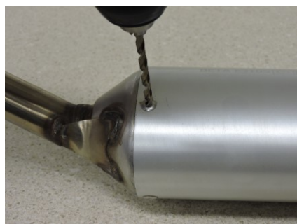
Figure 1- Pop rivet drilling.
