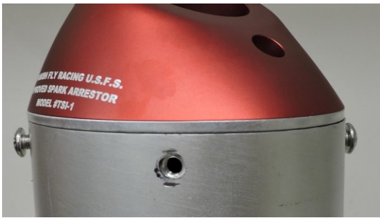
Figure 3-Checking screw hole locations in Can.
