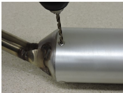
Figure 1- Pop rivet drilling.
