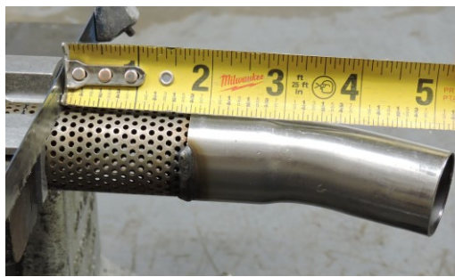
Figure 4-Perforated Tube rough cut location.
