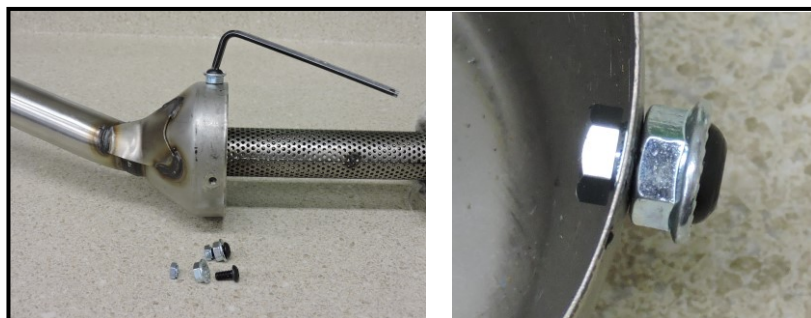
Figure 2- Installation of press in nuts into Inlet Cap.
