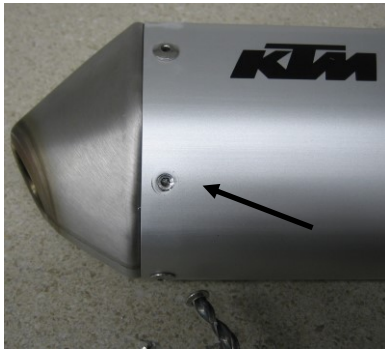
Figure 1 -Pop rivet head drilled out.
