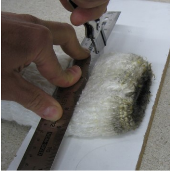
Figure 5 -Box knife cutting of silencer Packing. Figure 6 -Checking screw hole locations in Can.
