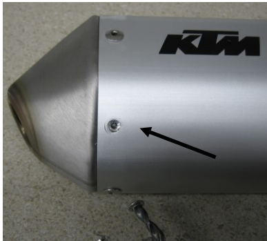
Figure 1 -Pop rivet head drilled out.
