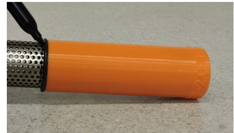
Figure 4 -Sharpie marking cut location.
