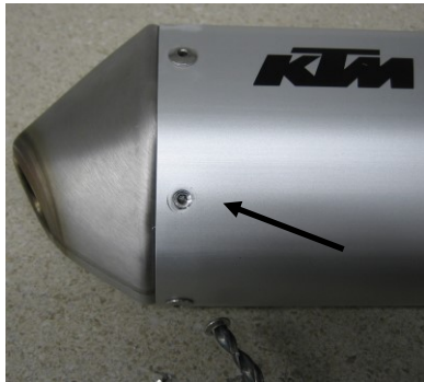
Figure 1- Pop rivet head drilled out.
