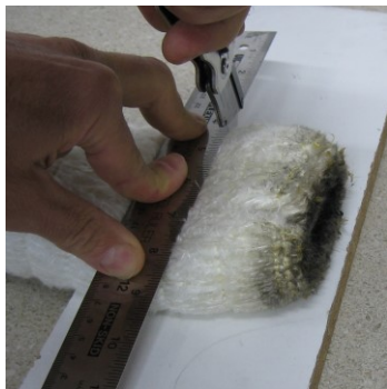
Figure 5-Box knife cutting of silencer Packing.
