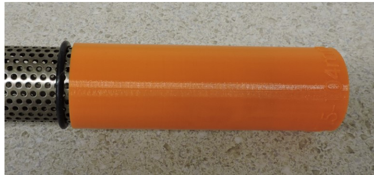
Figure 2- O- ring & measurement tool installed on Perforated Tube.
