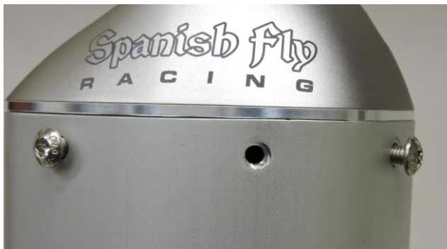
Figure 6-Checking screw hole locations in Can.
