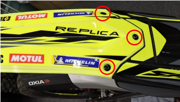
Figure 1 -Rear fender screw locations.
