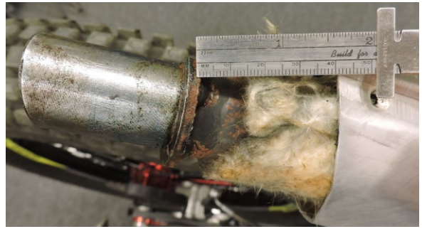
Figure 6- Measurement of stop plate to end of silencer.
