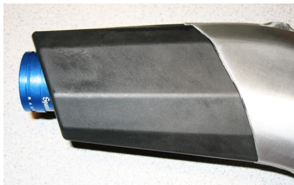
Figure 8 – Left side view of silencer body showing installed spark arrester.
