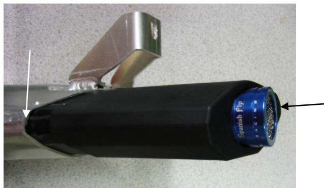
Figure 7 – Bottom view of end cap first entering silencer body (white arrow), and tapping location (black arrow).
