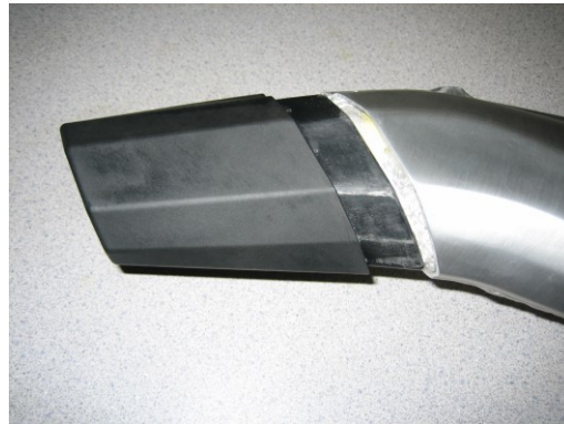
Figure 2 – View of end cap just separated from silencer body.
