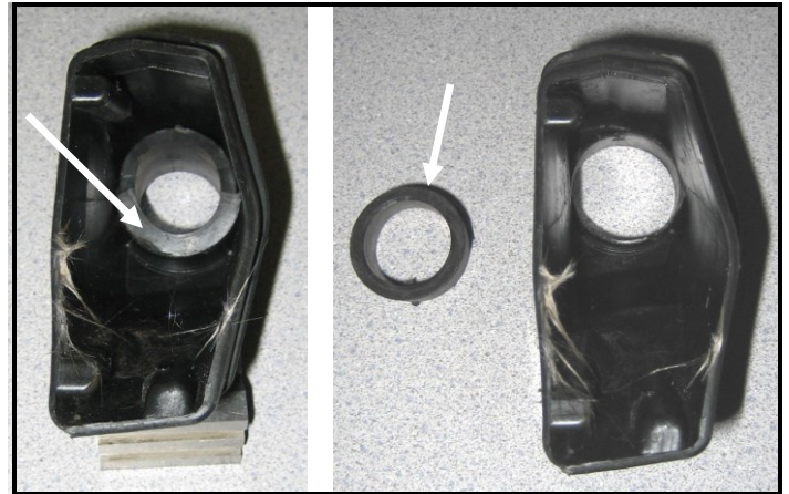
Figure 2- White arrow identifies rubber grommet installed (Left) & removed from end cap (Right).
