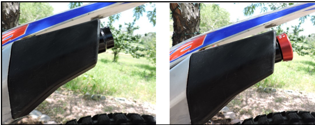
Figure 6 -Adapter installed (Left), adapter installed with TRS-1 spark arrestor (Right).
