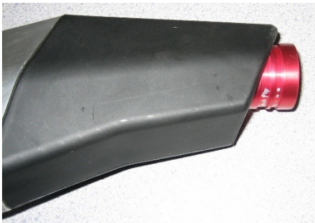
Figure 7 – Left side view of silencer body showing installed spark arrester.
