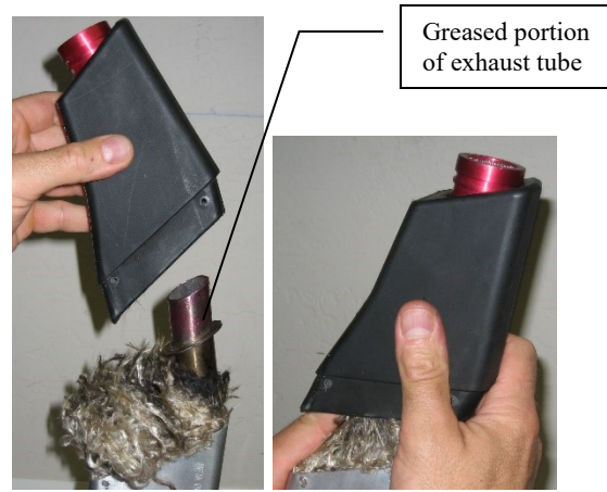
Figure 6 – End cap being installed onto silencer body, note exhaust tube is directed to the I.D. of the spark arrester.
