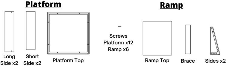
Insert Long and Short Sides into slots in Platform Top and secure with (8) screws with provided wrench
