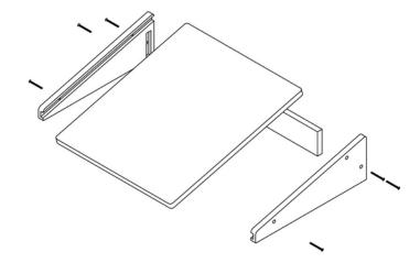
Insert Ramp Top and Brace into slots in one of the Side pieces and secure with (3) screws.
