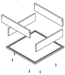
Secure Long and Short Sides together with (4) screws
