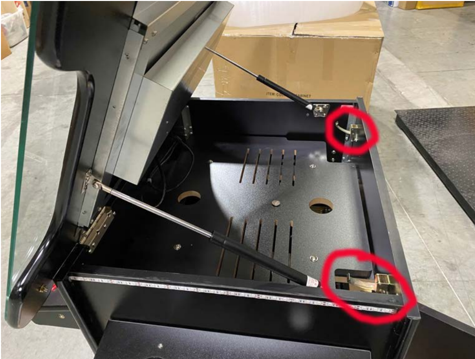
Here is a view of the latches from the top side of the machine
