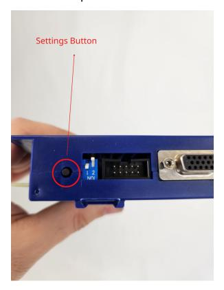
• Power the arcade back on and allow it to load. Text will appear prompting you to press the settings button.
