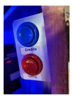
In all other models, open the back door of the arcade using your key and press the settings button located on the game box near the dip switches and video input
