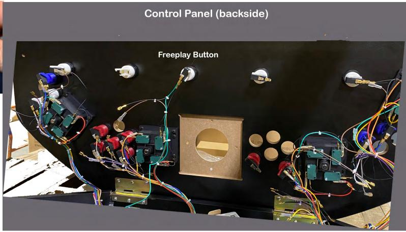
Once you loosen those bolts, you should be able to lift up on the control panel and have it open up to show you the backside. Once there, disconnect the green wire connected to the freeplay button.
