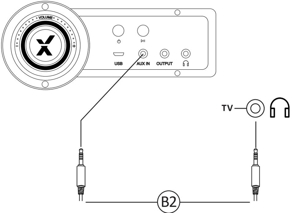
1. Connect **B2** cable to X Rocker control panel 3.5mm INPUT socket.
