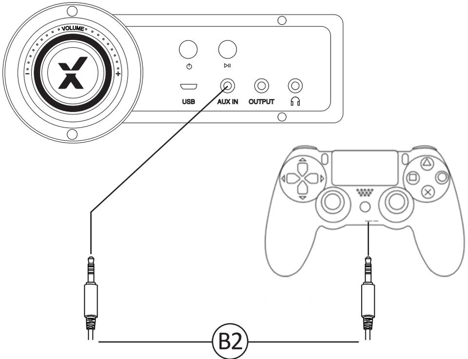
1. Connect the **B2** cable to the bottom of the PS4 controller via the headset socket.
