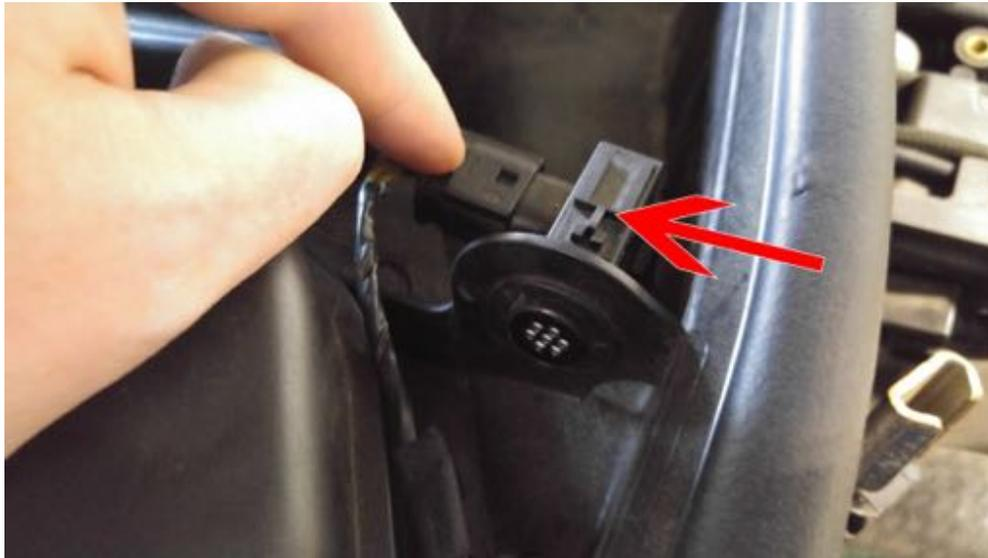
There is no need to remove the sensor, just unclip the wire from it and move the rest of the wire out of your way.
