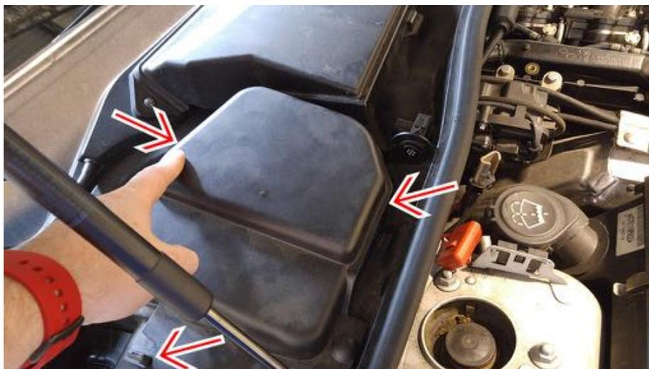
The three arrows point to the three clips that have to be undone to remove this piece. The two hidden ones need to be pulled away from cover, the last one (lowest in picture ) just comes out of its slot. Once this is done lift it off and set it aside.
