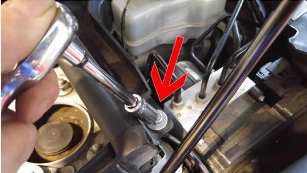
Next remove the 10mm bolts holding the cowl support down on either side. When this is complete lift the cowl out of the car and set aside.
