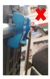
5. Caution! Do not over tighten the mounting screws. Using a power drill may cause damage, hand tighten only. Using the provided Torx key, tighten the screws until they are snug, then turn them another ½ turn. Check periodically for tightness.
