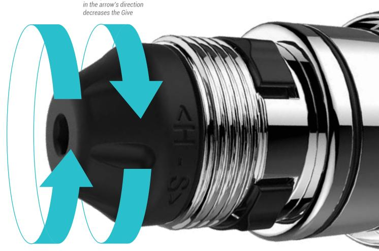
Turning the Give Knob in the arrow's direction increases the Give or locks it completely. Always back one click from maximum settings
