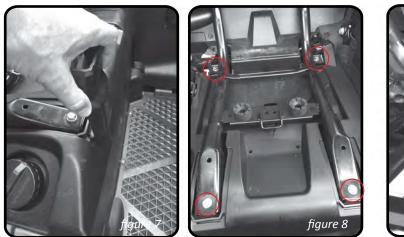
**STEP 7** Remove the two rear and two front nuts as indicated and lift out passenger seat (*figure 8*).
