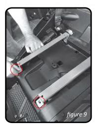
**STEP 9** Re-install the 2 front OEM nuts removed in Step 7.
