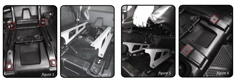
**STEP 3** Install driver side angle brackets. Position as shown *(figure 2)*, and re-install nuts removed in step 2.
