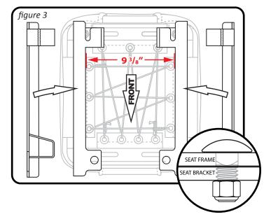
**STEP 4** Install the left and right passenger seat brackets as shown. Brackets should be spaced apart 9 <sup>3</sup>/8", centered on the seat frame. Secure with four nyloc nuts (*figure 3*).
