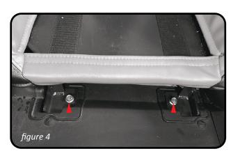
**STEP 6** Remove the driver seat bottom by pulling up on the front of the seat pan. Set aside. Using a 12mm socket, remove the four frame bolts as shown and remove frame assembly. NOTE: Retain these bolts for future use (figure 5).
