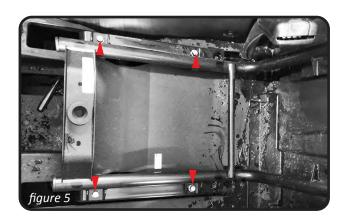
**STEP 7** Attach the driver-side seat brackets to your ADS-1 seat as shown, using four nyloc nuts. **NOTE:** the laser cut arrows should point at the front of the seat and the slotted sections face the sides of the seat. Brackets should be positioned 8 1/2" apart and centered on the seat (*figure 6*).
