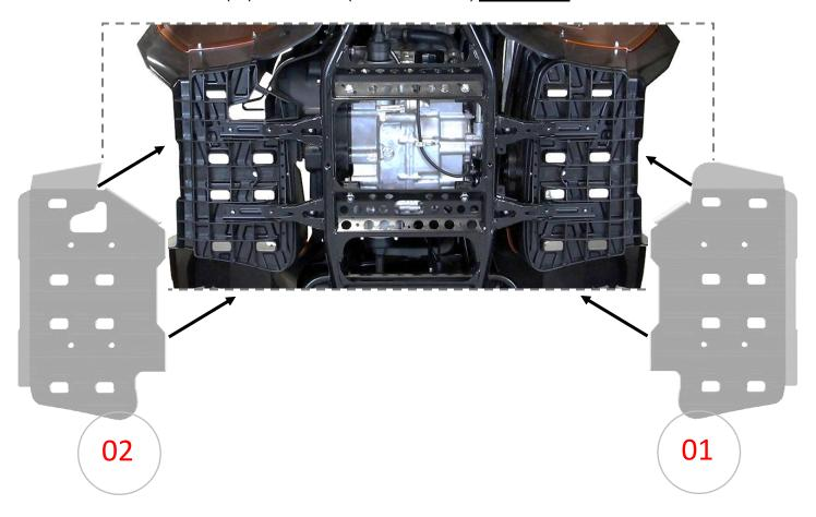
5. Secure the floorboard using (4x) M6 fender washers and (4x) M6-1.00 lock nuts for each side.
