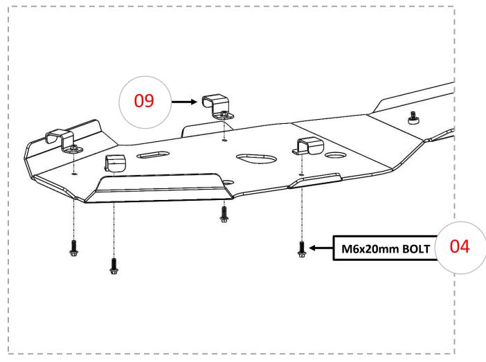
5. Using the provided steel clamps, secure the front to the frame. Refer to the schema below.
