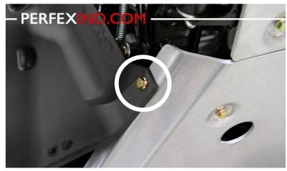
7. Once both skid plates are correctly installed, tight all the bolts appropriately.
