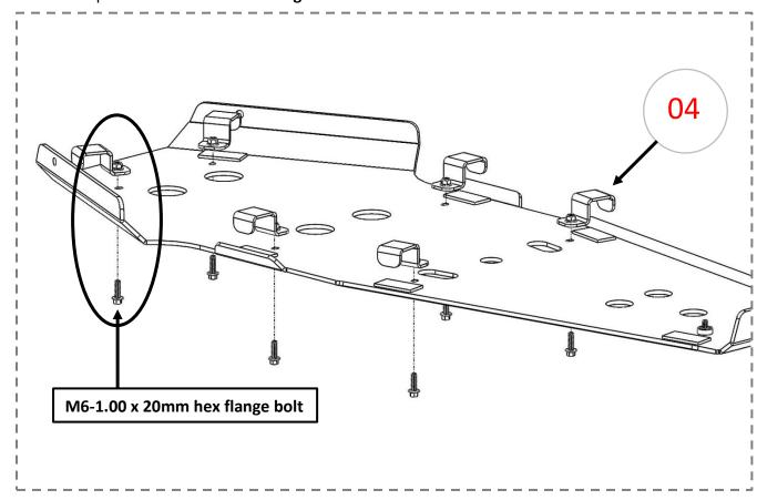
3. Install the front skid plate to the frame. Use (2x) M6-1.00 x 40mm hex flange bolt, (2x) 3/4" Lg. spacer, (2x) 1/4" fender washer and (2x) M6-1.00 lock nut. See image below.
