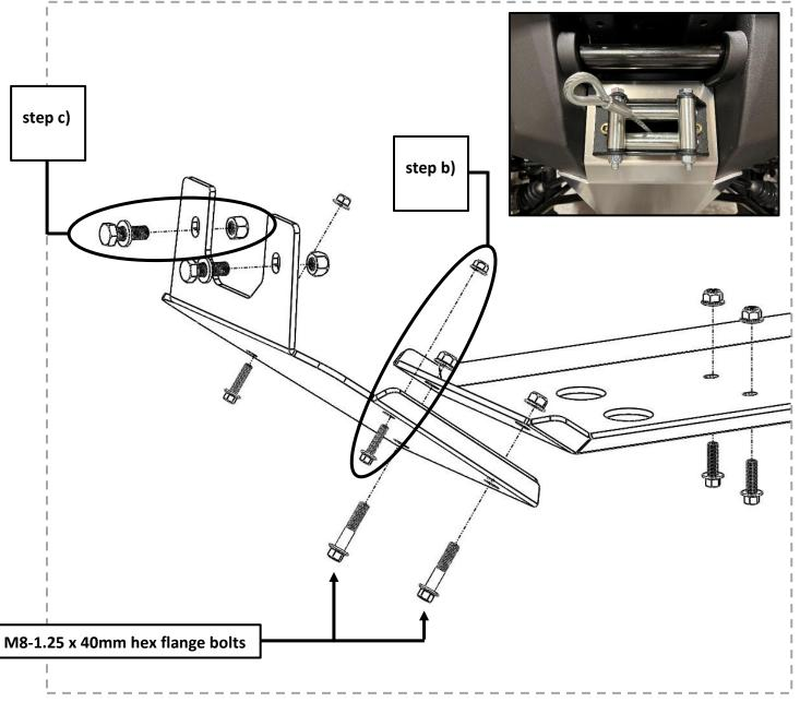
8. Once the 3 plates are correctly installed, tight all the bolts appropriately.
