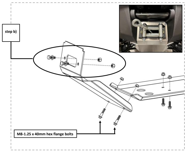
10. Once the 3 plates are correctly installed, tight all the bolts appropriately.
