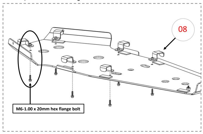
3. Install the front skid plate to the frame. Use (2x) 1-1/4" clamp and (2x) M6-1.00 x 20mm hex flange bolt. See image below.
