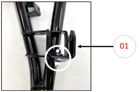
2. Install the bracket to the shock mount using (1x) M10x70mm bolt, (1x) 1-1/4" Lg. spacer and (1x) M10 lock nut. **Note:** Put the spacer inside of the shock mount.
