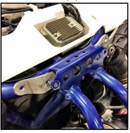
2. Then, insert the second front bracket (01) outside of the frame shock mount. Use M10-1.50 x 60mm hex bolts, 1-1/8" Lg. bushings and M10-1.50 lock nuts. See image below.
