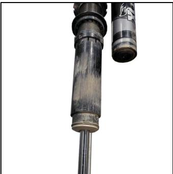
4. Insert the lift spacer (03) on the shock.
