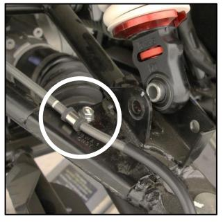
• Rotate de clamps on the other side and reinstall using factory bolts. See image above
