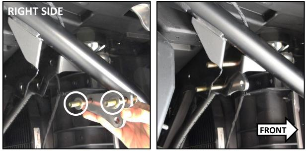
6. Use (1) 1-3/16 Lg. spacer on each bolt, inside of the shock mount.
