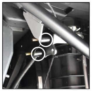
7. Insert (1) M10 heavy washer at the end of each bolt.
