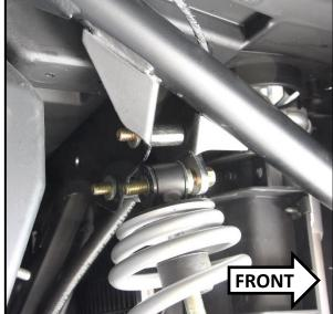
10. Insert (2) M10 heavy washer at the end of the bolt.
