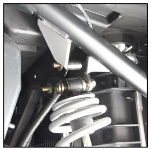
11. Insert (1) front bracket to the assembly. Secure each bolt using (3) M10-1.50 nylon nut. Tight completely all the hardware appropriately at this point (don't forget the bottom of the shock).
