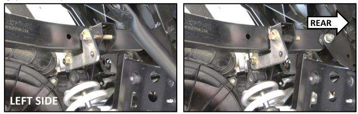
2. Insert (1) rear bracket to the assembly. Secure each bolt using (2) M10-1.50 nylon nut. Don't tight completely at this point.
