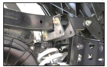
3. Connect the top of the shock to the brackets. Use (1) M10-1.50 x 65mm bolt, (2) M10 heavy washer and (1) M10-1.50 nylon nut. Put one washer on each side of the shock eyelet. Tight all the hardware completely at this point.
