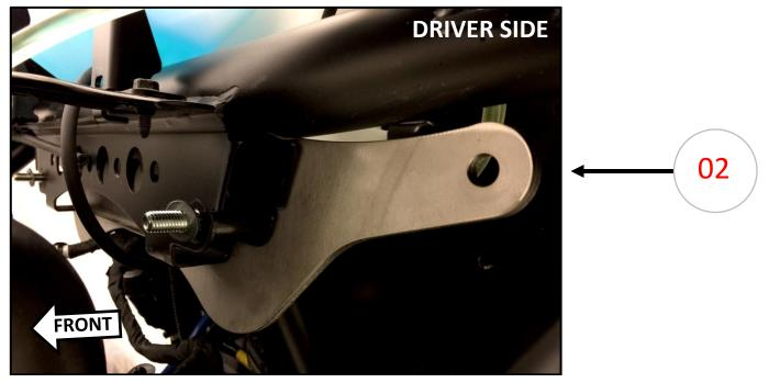
2. Insert the second bracket (01) to the assembly. Secure with M10-1.50 lock nuts at the end of each bolt.
