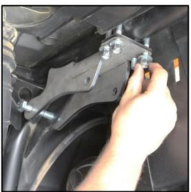
4. Secure the bracket to the shock mount using **(2) M12 washer**, **(1) 1-3/16" Lg. spacer** and **(1) M12-1.75 nylon nut**. Put the washer between the frame and the bracket, both sides. And the spacer inside of the shock mount.
