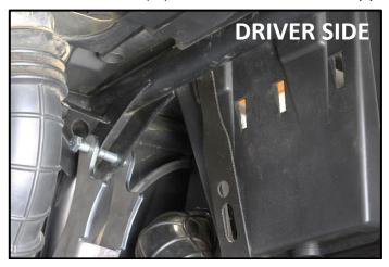
2. Insert (2) U-Bolt to the frame, as shown below.
