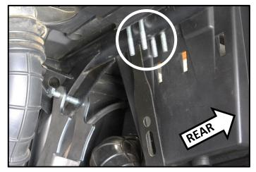
3. Secure the bracket to the U-Bolts using (4) M10 washer and (4) 3/8"-16 nylon nut. Do not tight completely.
