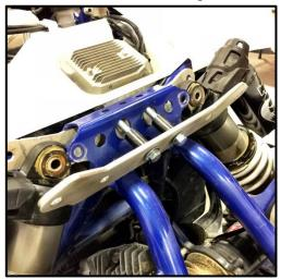
3. Install the brackets to the frame shock mount. Use M10-1.50 x 65mm bolts, 1" Lg. bushings and M10-1.50 lock nuts.
