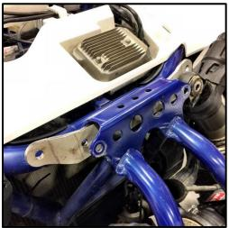
2. Then, insert the second front bracket (01) outside of the frame shock mount. Use M10-1.50 x 60mm hex bolts, 1-1/8" Lg. bushings and M10-1.50 lock nuts. See image below.
