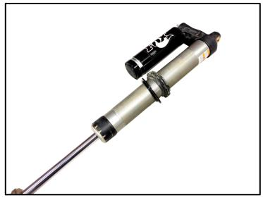
4. Insert the lift spacer (03) on the shock.
