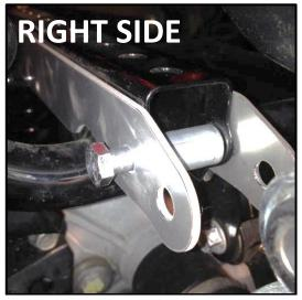
2. Connect the top of the shocks to the brackets. Use M10-1.50 x 60mm bolts, M10 washers and M10-1.50 lock nuts. Put one washer on each side of the shocks eyelet.
