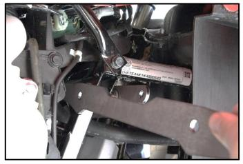
4. Secure using M10-1.50 lock nuts.
