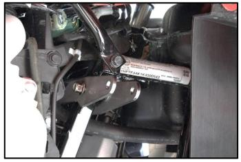
5. Connect the top of the shock to the bracket assembly. Use M10-1.50 x 55mm bolts, 10mm ID. x 3/16" Lg. spacers and M10-1.50 lock nuts. Put one spacer on each side of the shock eyelet.
