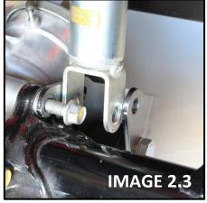
3. Connect the bottom of the shock to the new shock location on the bracket. Use M12-1.75 x 65mm bolt, M12 washer, big spacer and M12-1.75 lock nut. Put the spacer between the shock eyelet.
