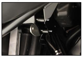
3. Insert another one front bracket to the assembly, inside of the shock mount.
