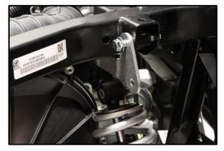
3. Insert another one rear bracket to the assembly, inside of the shock mount.
