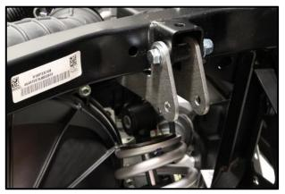
5. Connect the top of the shock using the factory hardware.
