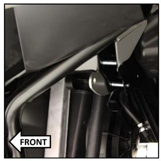
2. Insert one spacer on each bolt, inside of the shock mount.
