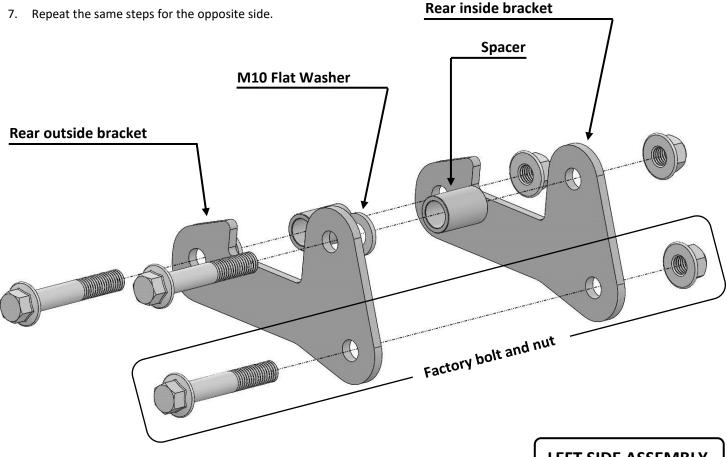
8. Once both sides will be completed, remove the factory nuts that they are into the factory rubbers (4x). Discard factory nuts.
