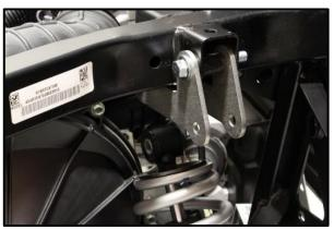
4. Secure with 2 M10-1.50 lock nuts. Don't tight completely at this point.
