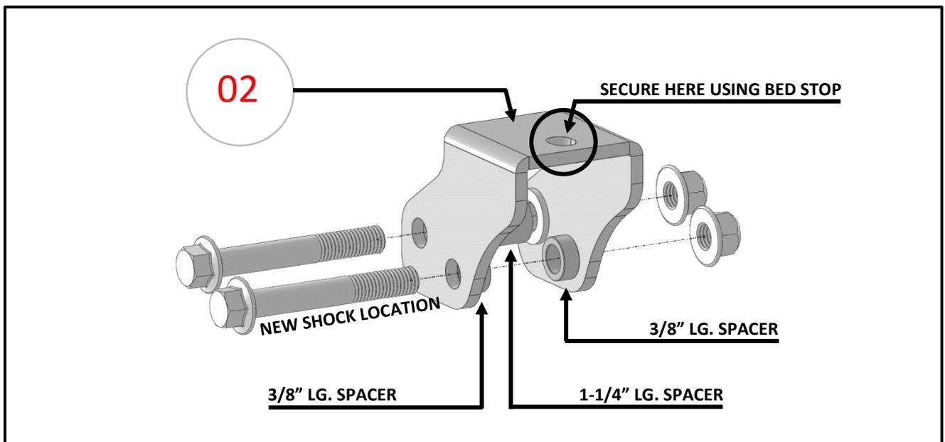
4. Tight all the hardware appropriately at this point. Use a 19mm wrench and socket.
