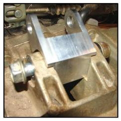
2. Connect the bottom of the shock the bracket. Use M12-1.75 x 75mm bolt and M12-1.75 lock nut. Torque the nut to factory specification.
