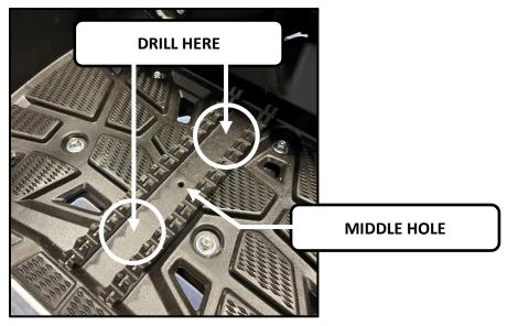
Install the foot pegs using, for each side: (2x) M8x40mm bolts, (2x) 5/8" bushings, (2x) M8 washers and (2x) M8 lock nuts. Refer schema below.
