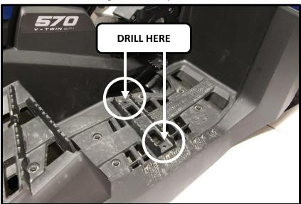
2. Install the foot pegs using, for each side: (2x) M8x40mm bolts, (2x) 9/16" bushings, (2x) M8 washers and (2x) M8 lock nuts. Refer schema below.
