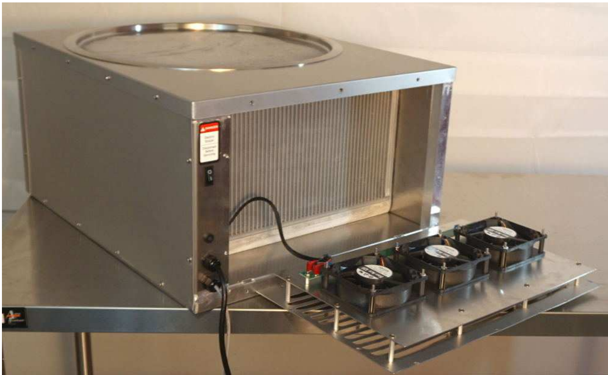
Figure 9: Fan panel removal
