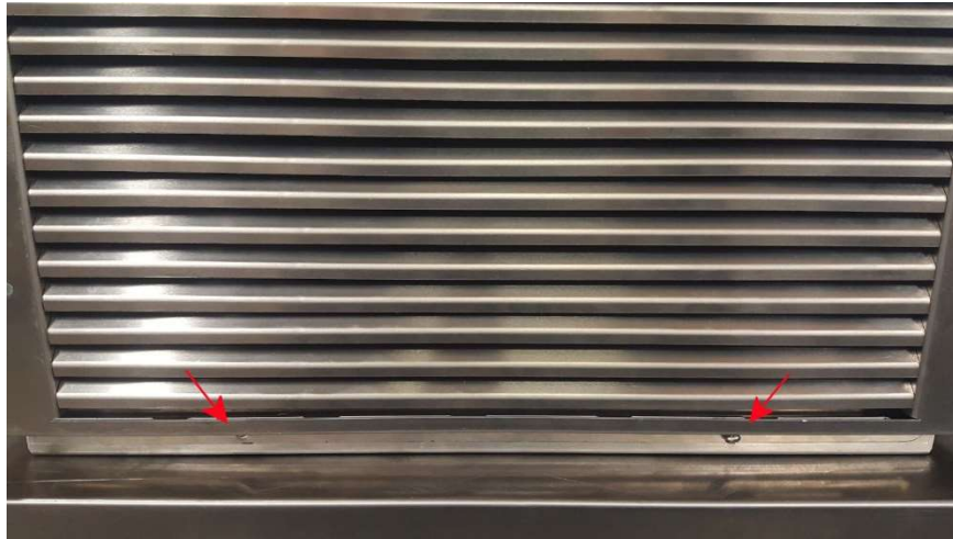
Figure 8: Fan cover panel screw removal
