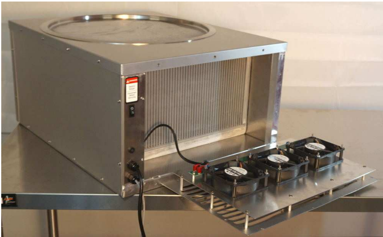
Figure 10: Fan panel removal
