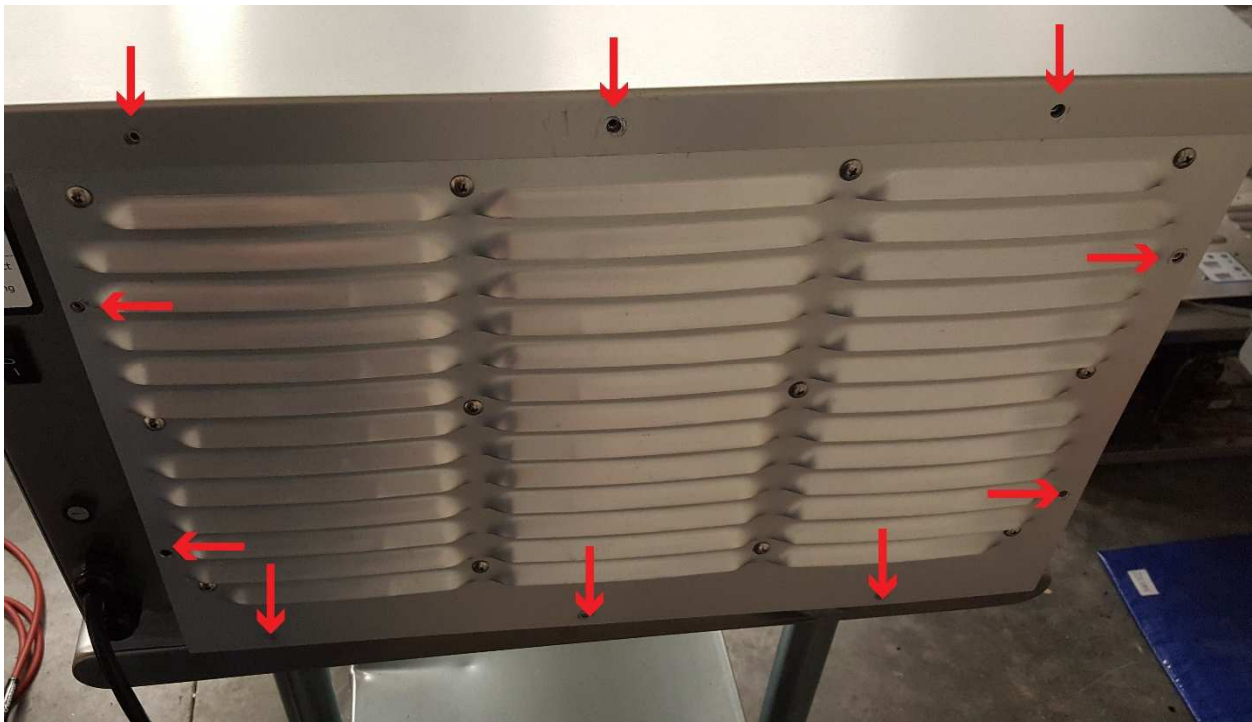
Figure 9: Fan panel screw removal
