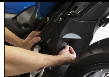
5 Apply a small amount of Loctite 248 to the M6 Screw. Hold the MudSling in position and thread screw into the Coupling Nut finger-tight.
