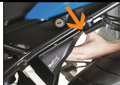
4 Place MudSling above rear tire and under the existing fender. Locate the MudSling wings against the registration point (welded feature on frame).
