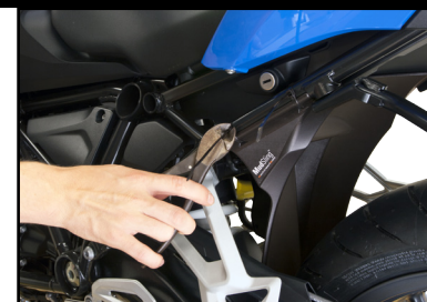
8 Cut off excess zip tie length with a side cutter for best appearance.
