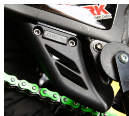
2 x C/Sunk Bolts M6x10 - 10Nm 2 x Bolts & Washers M6x20 - 10Nm
