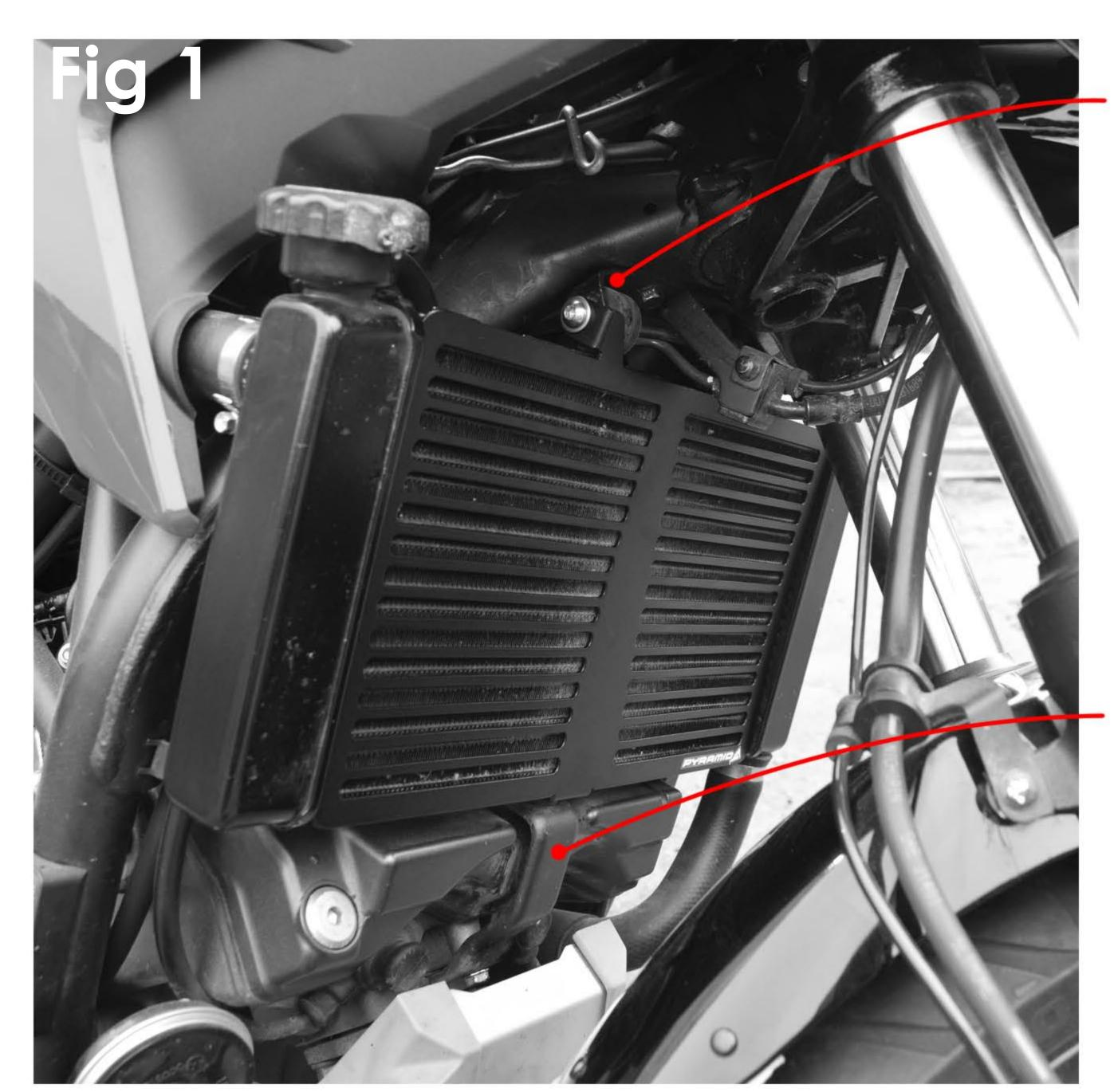
Remove the bolts on each side at the top of the radiator guard
