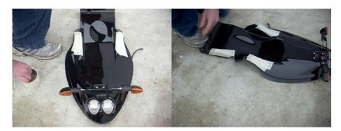
Feed the undertray in from rear of bike (keep electronics held out of the way)
