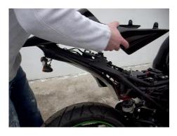
Stand back and check that the undertray is inside the seat unit looking from the rear of the bike.
