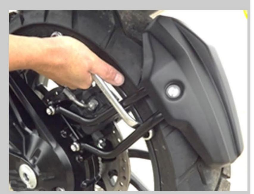
Once finished spin the wheel and check the guard isn't fouling on the wheel or tyre and to make sure the bolts aren't catching on the face of the brake disk.
