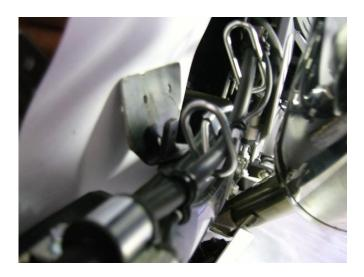
using the M6 x 20mm bolt supplied, refit the brake hose guide to the tab, fully tightening the bolt, which should pass through the single hole in the bracket. Secure the bracket to the tab with the Nyloc nut and steel washer supplied to the rear of the bracket. Fully tighten.
