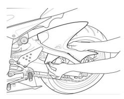
**4** Secure the hugger in place using the Three original fixing points and bolts removed in step 1.
