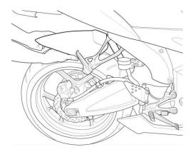
**3.**From the rear of the bike, slide the hugger over and around the wheel as shown.
