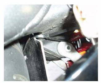
**6.** Fix the lower protection arm away from the tyre using the zip tie provided.
