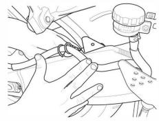
Using the original bolt, secure the mounting bracket **between** the brake line holder and the swinging arm.
